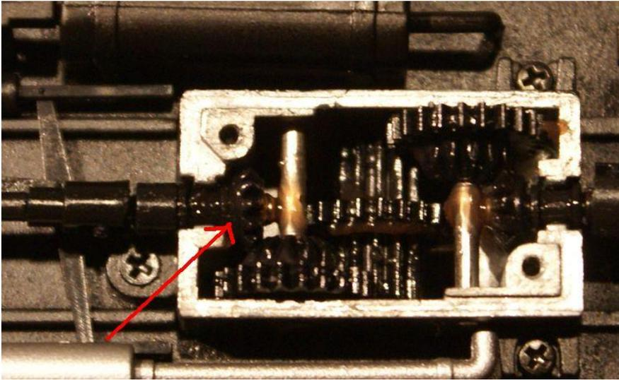
Replace the drive line with the parts indicated with the red arrow in the first picture. Replace the wheels and cover, and reattach screws.
