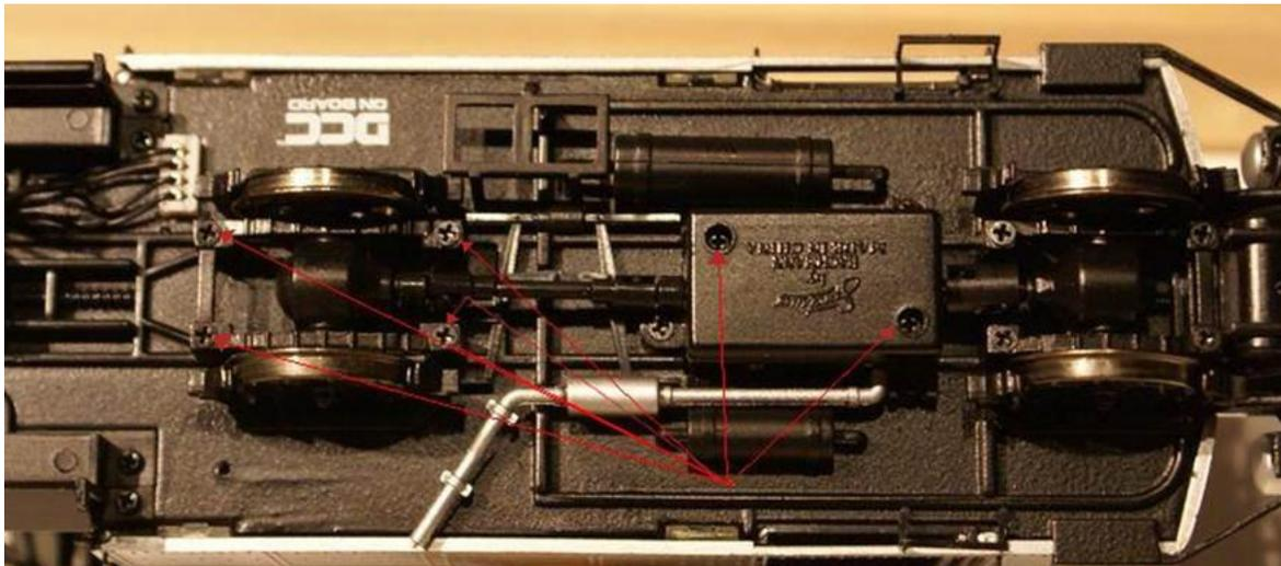
Remove the rear wheel and the drive line. Gently try to spin the gears on the shaft with your finger. The split gears will spin freely.
